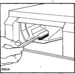
After each wash programme, partially pull out the detergent drawer to let it dry. The filter collects fluff and any small objects which may accidentally have been left in the laundry.
