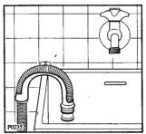
**Joined into a branch of the sink waste pipe.** The branch must be above the sink trap and at least 60 cm above the floor.
